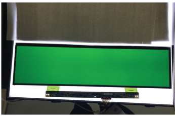
图 5 倒置 U 型面板点屏图片 Fig.5 Picture of inverted U-type TFT panel
